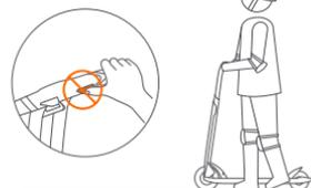
⚠ DO NOT press the throttle when walking with the KickScooter.
