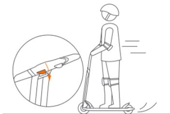
3. Slow down by releasing the throttle. To stop, press the electric brake and stamp the fender at the same time to trigger mechanical braking.
