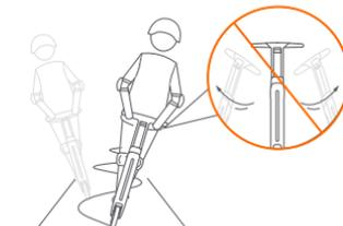
⚠ DO NOT rotate the handle violently while driving at high speed.
